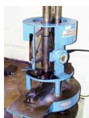
Impact Sensitiveness (Rotter Impact Machine)
