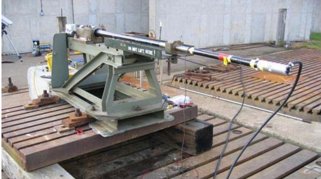
Figure 3: 30mm calibre, alternative lower velocity gun system
