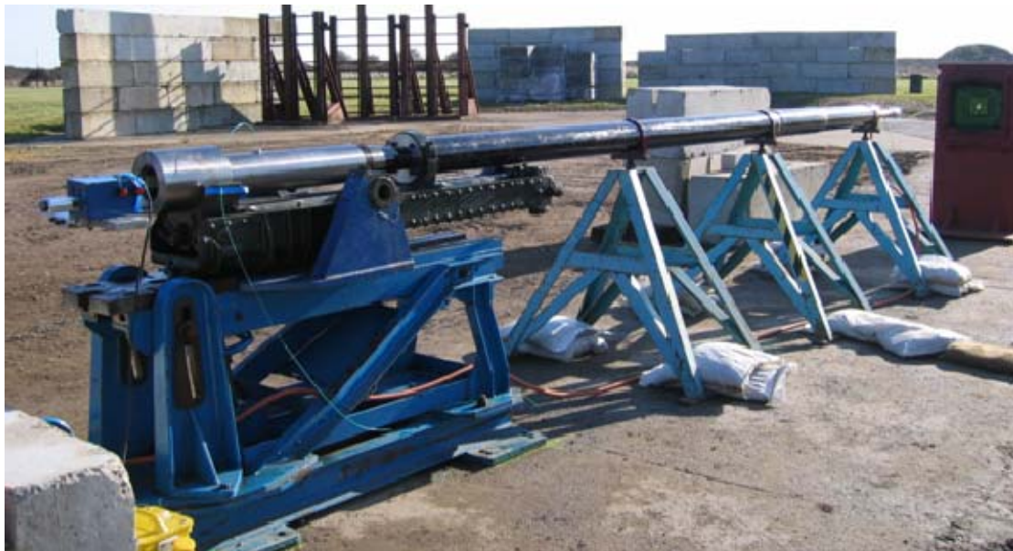
Figure 2: 40mm calibre, 6.6m long high velocity gun system
