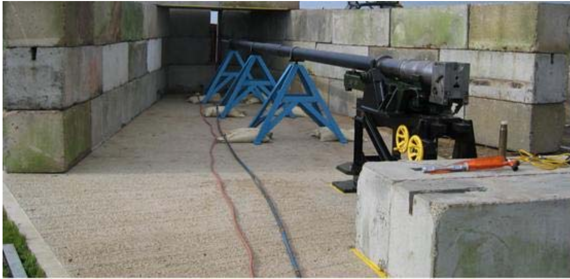
Figure 1: 40mm calibre, 10 m long high velocity gun system
