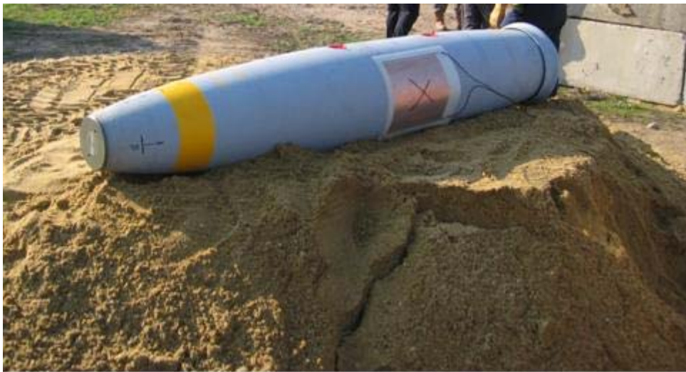
Figure 7: Raytheon Precision Guided Bomb prior to the high velocity STANAG 4496 test
