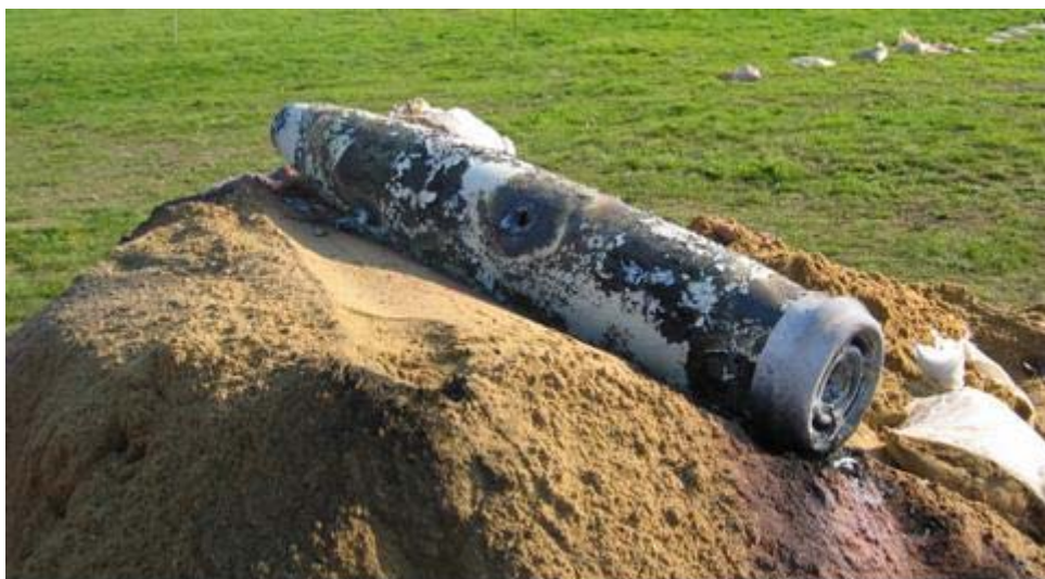
Figure 8: Raytheon Precision Guided bomb after a cooling off period showing IM compliance from the high velocity STANAG 4496 test.
