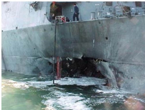
Figure 1 – Damage to USS Cole at Aden
