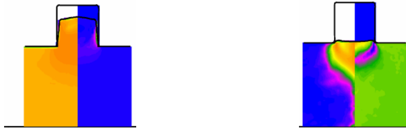
Figure 15: Simulations of PBXN109 above (L) and below (R) rise rate threshold showing damage
