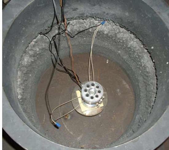
Figure 2: Assembled test fixture in the chamber ready for testing.
