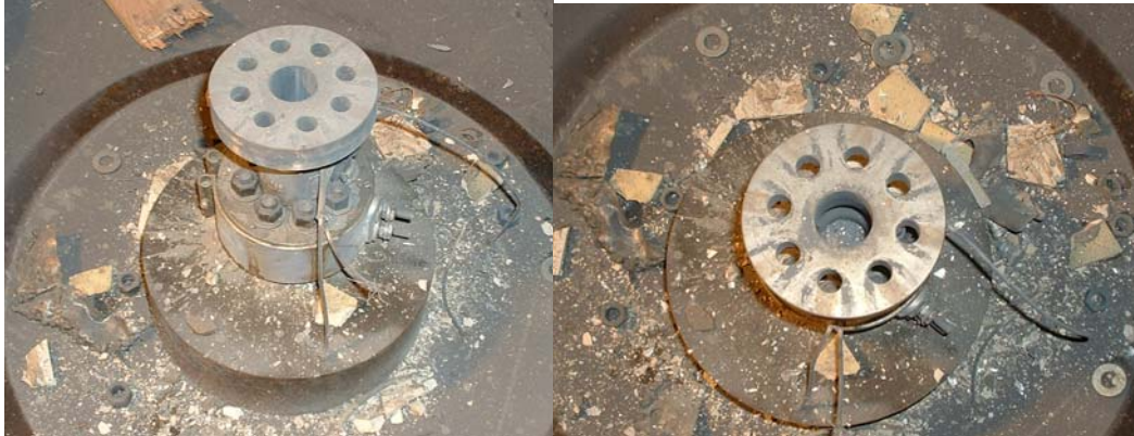
Figure 7. 5.1mm diameter vent test result for PAX-28.
