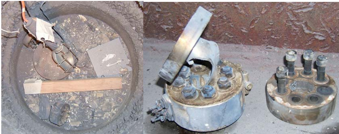
Figure 8. 6.4mm diameter vent test result for PAX-28.
